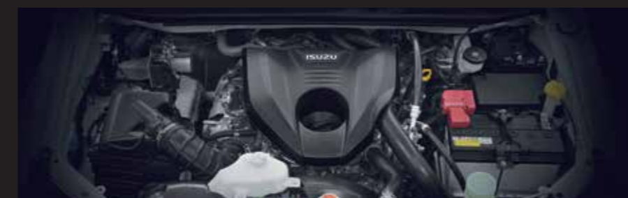
ISUZU 4JJ3 3.0L Engine with Max Power 190PS @ 3600 rpm / Max Torque 450 Nm @ 1,600 - 2,600 rpm
